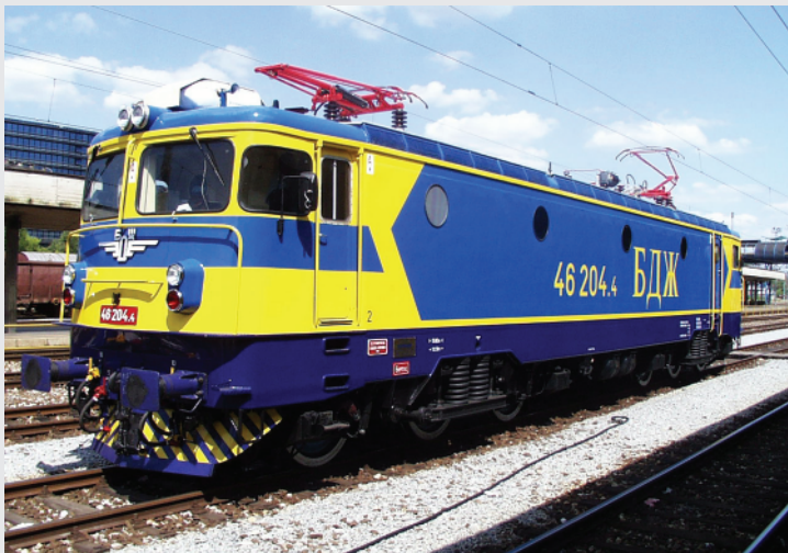
Thyristorized Co'Co' locomotive for Bulgarian Railways
