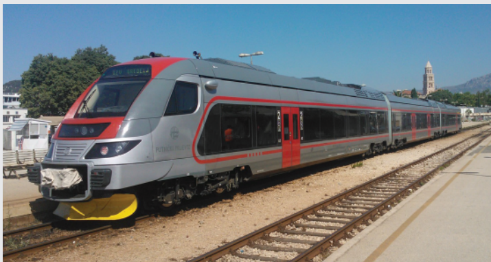
Diesel-electric multiple unit for Croatian Railways
