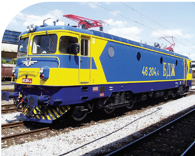
Thyristorized Co'Co' locomotive for Bulgarian Railways
